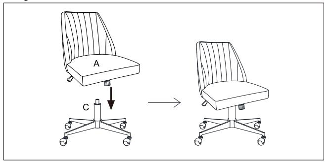
Position the Seat (A) over the top of Gas Lift (C). Insert the Gas Lift (C) into the center hole of Lift Mechanism (B) and press down until fully engaged.
