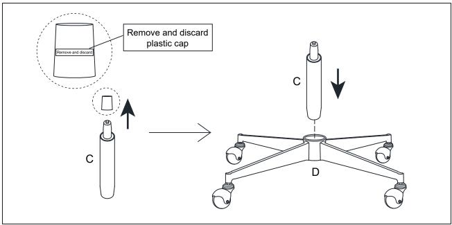
Remove and discard plastic cap from Gas Lift (C). Insert Gas Lift (C) into the center hole of Base (D) as shown.
