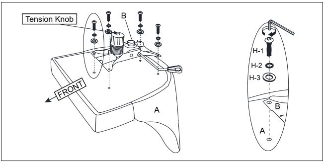
Align holes on Lift Mechanism (B) to pre-threaded holes on Seat (A). Attach Lift Mechanism (B) using Allen Bolts (H-1), Spring Washers (H-2) and Flat Washers (H-3), stacking hardware in the order as shown. Make sure the Tension Knob faces towards the front of chair assembly. Engage Allen Bolts (H-1) using Allen Key (T-1) but do not fully tighten until all 4 bolts are inserted into holes.
